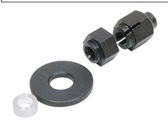
Jam nuts like these can prevent an engine from tossing the back plate, spinner, thrust washer, etc. A 4 stroke engine set to run too rich will cause the engine to run backwards and toss these engine parts. The YS engines and some Saito engines are notorious for suddenly running backwards during the startup and carb adjustment. Be careful! Putting carborundum sanding disks between the prop driver, the prop, back plate, and thrust washer can help,
