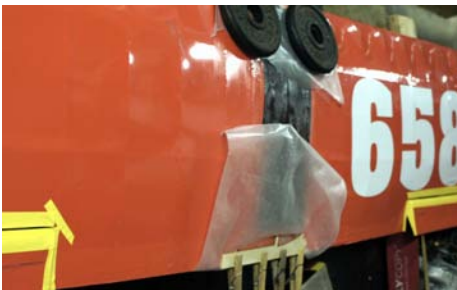
Top side of the wing —weights and clamps to hold the position of the wing halves.
