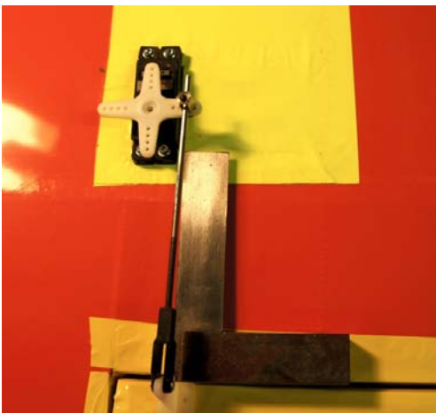
Push rods and control horn installed at 90 degrees
