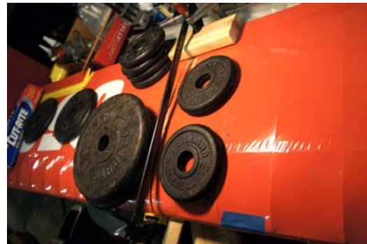
120 Minute epoxy was used to glue the dihedral braces with weights, clamps and two Robert Incidence meters used to hold the position of the wing halves.
