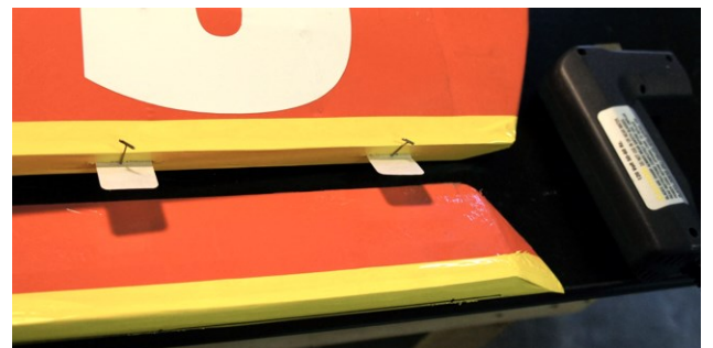
After covering the new wood, the hinge slot tool used to make slots and CA hinges installed. The pins help locate the center of the hinge and let the CA wick between sides.
